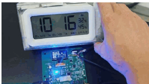
Hot-end functional photograph: +85^{\circ}\text{C} / 16 V, source p. 58.
