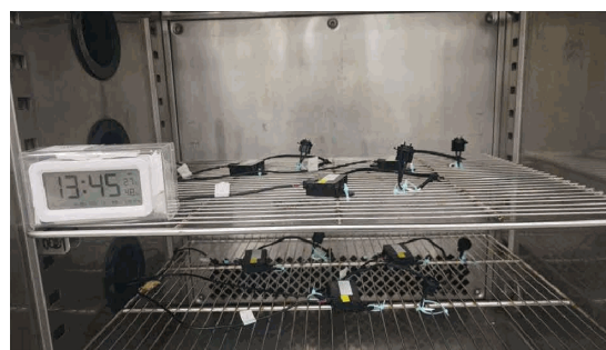
Figure A1 Original sample arrangement for temperature alternation.
