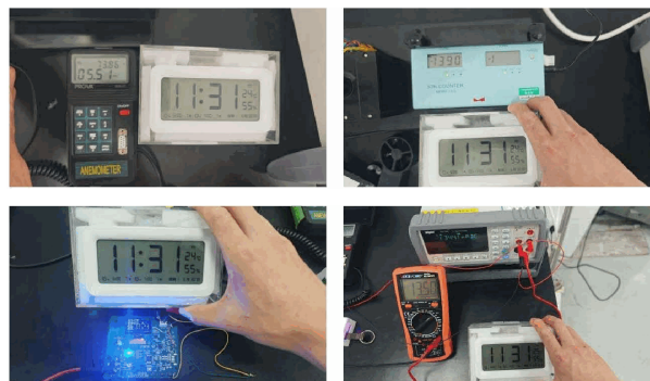
Figure B6 Original post-test check photographs, source pp. 60-61. Air-speed meter and ion counter above; module monitoring and electrical instruments below.
