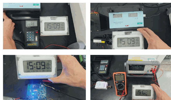
Figure 6 Original post-exposure bench photographs: airflow and ion-output measurement above; module monitoring and electrical checks below. Source p. 98.
