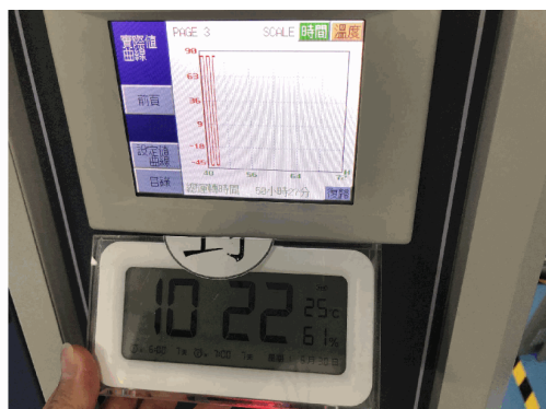
Figure 5 Original controller photograph showing the repeated hot/cold history.
