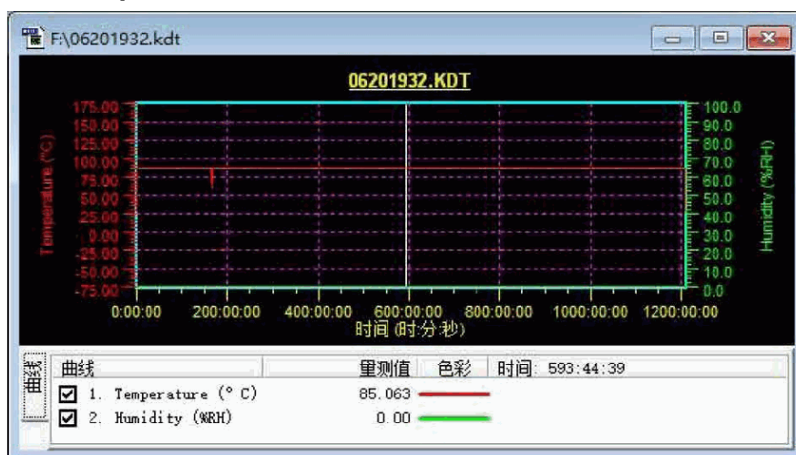
Figure 4 Original temperature-versus-time record. The horizontal axis extends to 1,200 hours; the red trace records chamber temperature during the high-temperature program.
