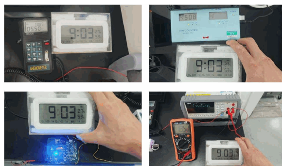
Figure 2 Original electrical, ion-output and monitoring checks after the test, source p. 49.
